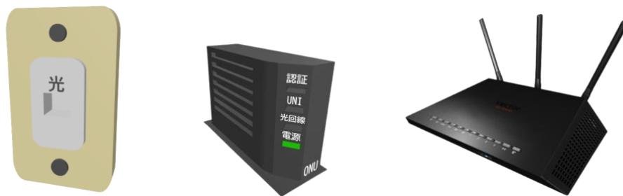
Figure 4 3D Models of Optical Outlet, ONU, and Wireless LAN Router
