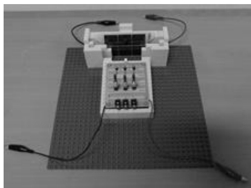
Fig.1 A photo of the demonstration set (a transmission circuit in the front side; and a solar panel as a receiver in the back side)
