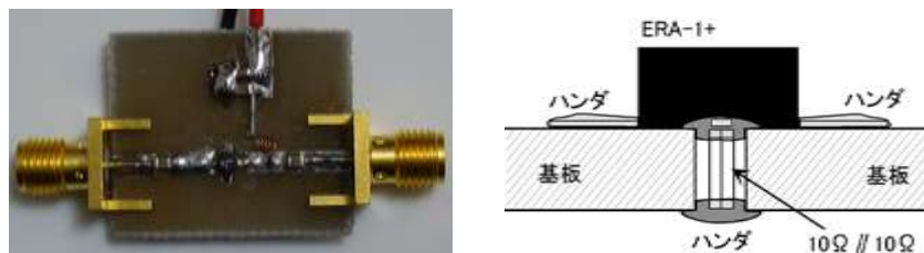
Fig.1 Photograph of the broadband amplifier and the structure of the feedback circuit.
