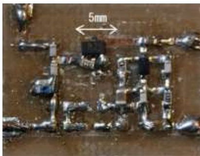
Fig 2. Photograph of the transistor mixer
