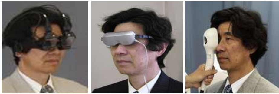
Fig.1 Image acquisition system of eye movement and papillary response by using goggle-type and handy-type of infrared CCD camera
