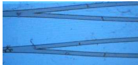
Fig. 2 Splitter waveguide patterns with 10 \mu\text{m} wide waveguides
