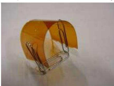
Fig.1 Appearance of flexible polyimide Optical waveguide
